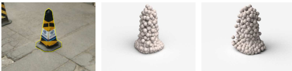
Figure 2.4: A point cloud reconstruction of a given 2D image visualized from two different views (Fan et al. (2017)) .
